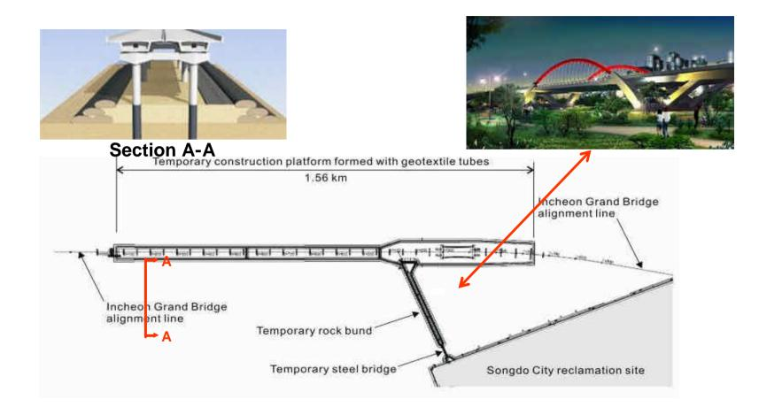
Plan view of geotextile tube artificial island
