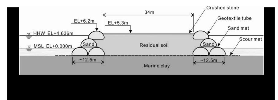
Typical cross section of Geotube<sup>®</sup> artificial island
